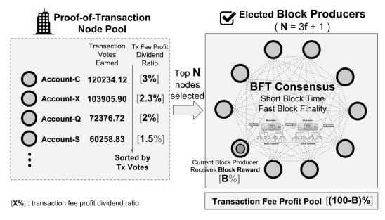
Figure 6.3 - Proof-of-Transaction based BFT blockchain consensus (public blockchain setup with no seed trust node)
